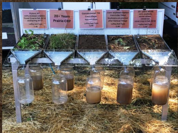
rainfall simulator in action, notice the difference in water clarity and infiltration with no-till and cover crops on left vs. conventional tillage and no cover crops on the right
