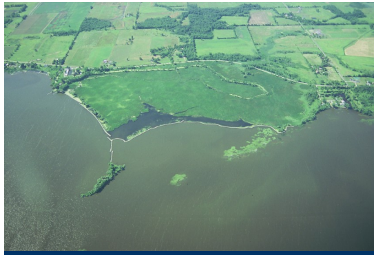
note the dark color behind the structure; this represents clear water compared to the dirty turbid water outside the structure
