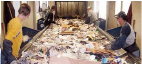
Pre-Sort Line: The sorters remove items that may harm or interfere with equipment such as plastic bags, large metal items and trash.
