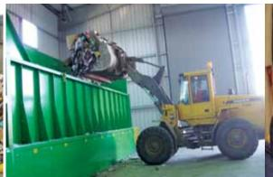
Metering Bin: This machine evenly meters the amount of recycling entering the facility.
