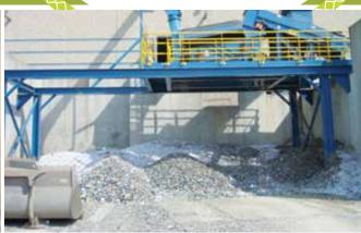
Glass Collection: Since glass is highly abrasive on conveyor belts and equipment, it is removed first and stored outside until it is shipped.
