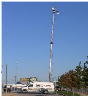
Exhibit 8-6 An example of a portable antenna
